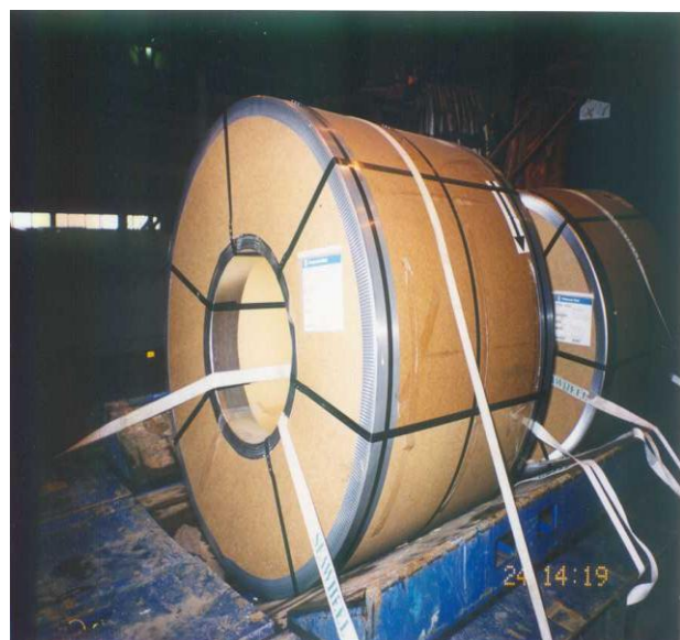
Straps through and across the coil
